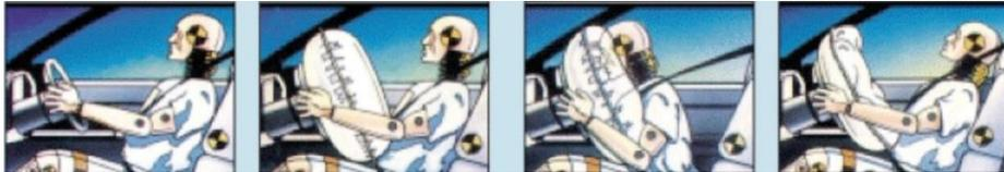
•Airbags supplement the seat belt by reducing the chance that the occupant’s head and upper body will strike some part of the vehicle interior. They also help reduce the risk of serious injury by distributing crash forces more evenly across the occupant’s body.
